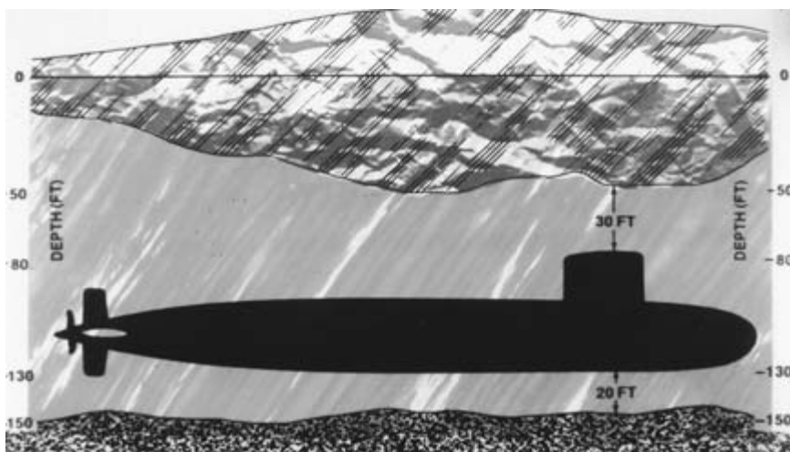
Figure 10.7 Artist's concept of USS Queenfish hugging bottom to avoid thick ice above it in shallow Chukchi Sea. (Courtesy of the U.S. Navy)
