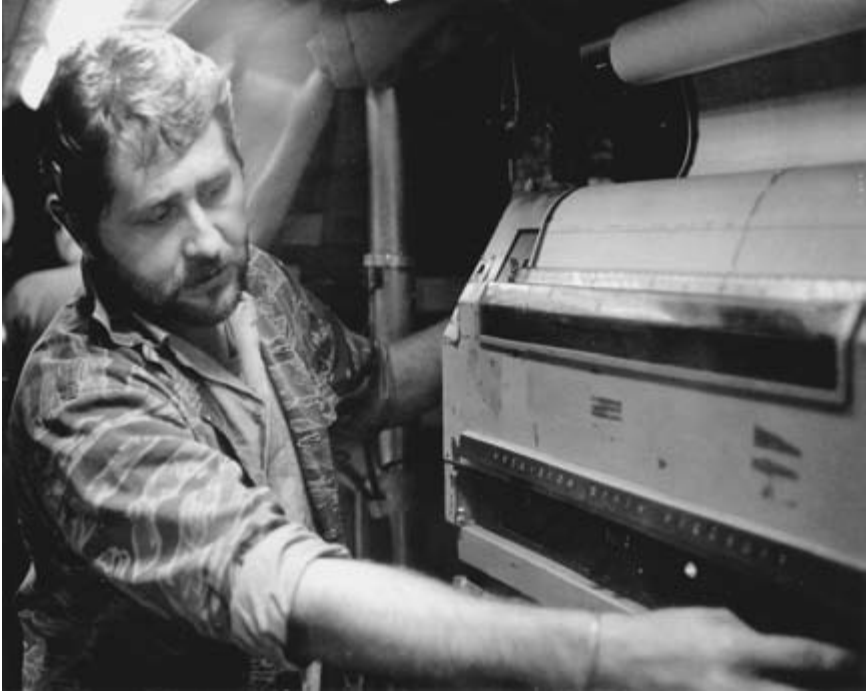
Figure 16.2 Quartermaster First Class Clarence F. Williams checking depth of water in Laptev Sea on precision depth recorder. (Courtesy of the U.S. Navy)
