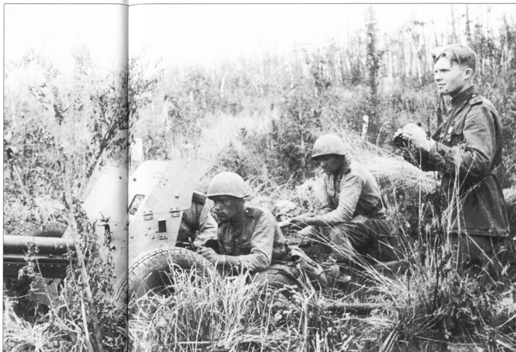
Ambush! A Red Army 45mm Model 37 anti-tank gun waits for its prey. It was a derivative of the German 37mm anti-tank gun but could fire high-explosive shells in an infantry support role.
