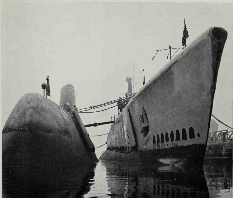
28. Nautilus moored alongside conventional submarine Greenling. Unusual shape of Nautilus' bow gives ship underwater speed and efficiency.
