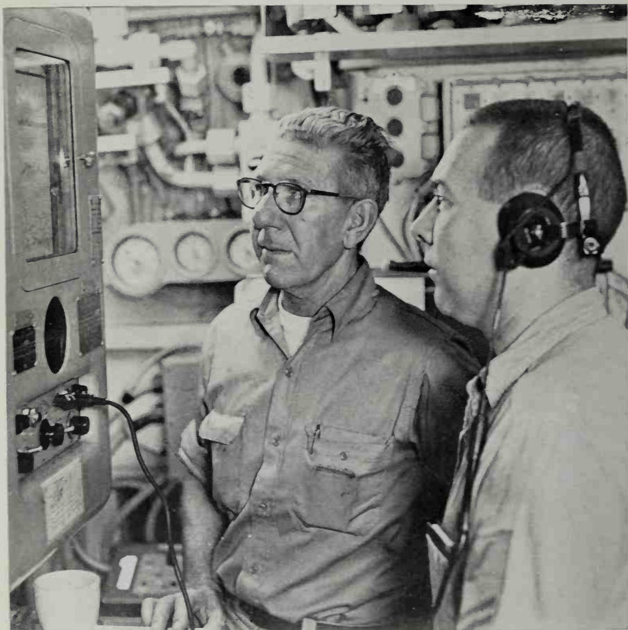
41. As Nautilus enters shoal water under ice, fathometer is constantly watched, for undersea mountains rise from the ocean floor.
