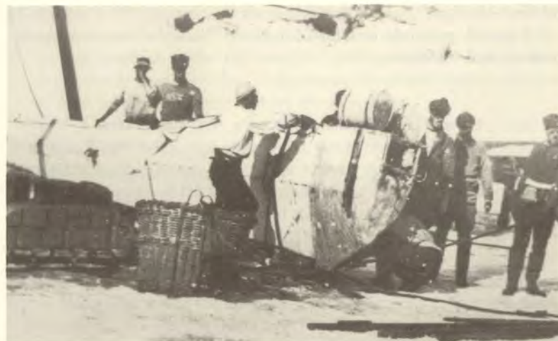
The R.E.P. Monoplane, minus wings, was used as an 'air sled' by the Mawson Expedition of 1911. (Author's collection)
