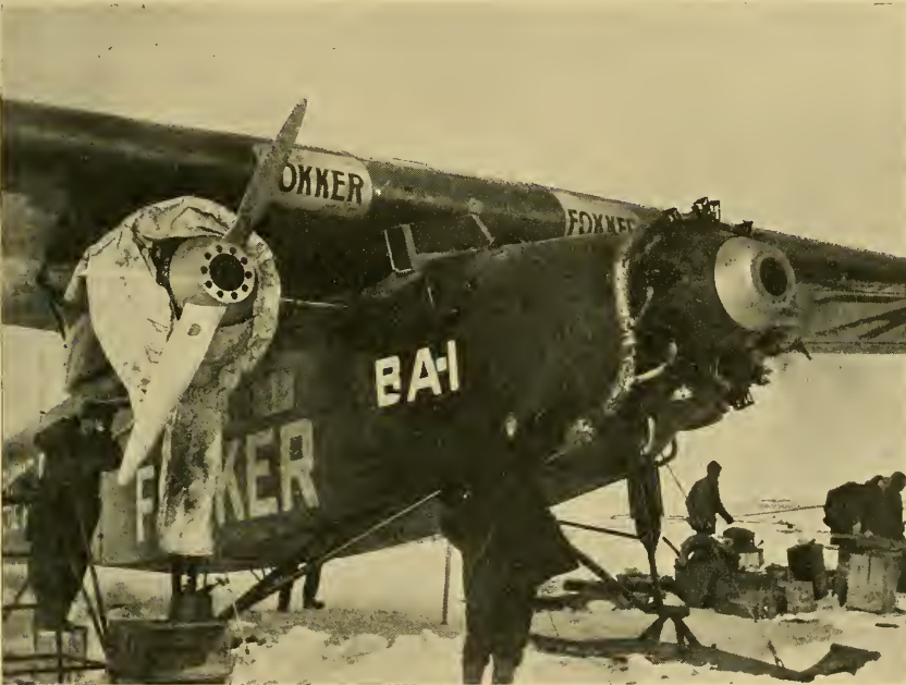
FIG. 1—The airplane used by the writer in the May 9, 1926, flight to the north pole showing, on the left, the fireproof canvas cylinder with pressure gasoline stove below used to heat the engine. On the right may be seen one of the skis used as landing gear. (Photograph copyrighted by Pathé News.)
