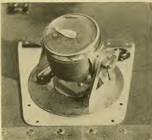
FIG. 3—A sun compass (Bumstead model) of the type used by the writer on the north polar flight. Note the shadow of the shadow pin on the pear-shaped hand of the 24-hour clock.
